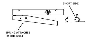
2) Diagram #2 shows the proper assembly order of spring and associated components.
